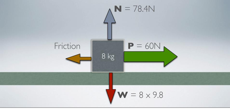
An 8kg block is pulled with a force of 60N over a rough surface where the coefficient of friction is 0.35. What is the acceleration of the block?
