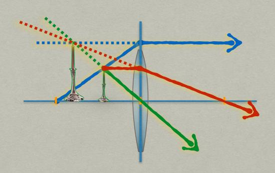
If the object is inside one focal length, a virtual image is formed and the magnification is positive
