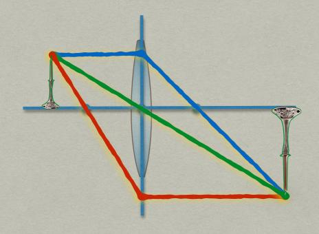
If the object is inside two focal lengths, the reverse occurs and thee magnification increases the size of the image
