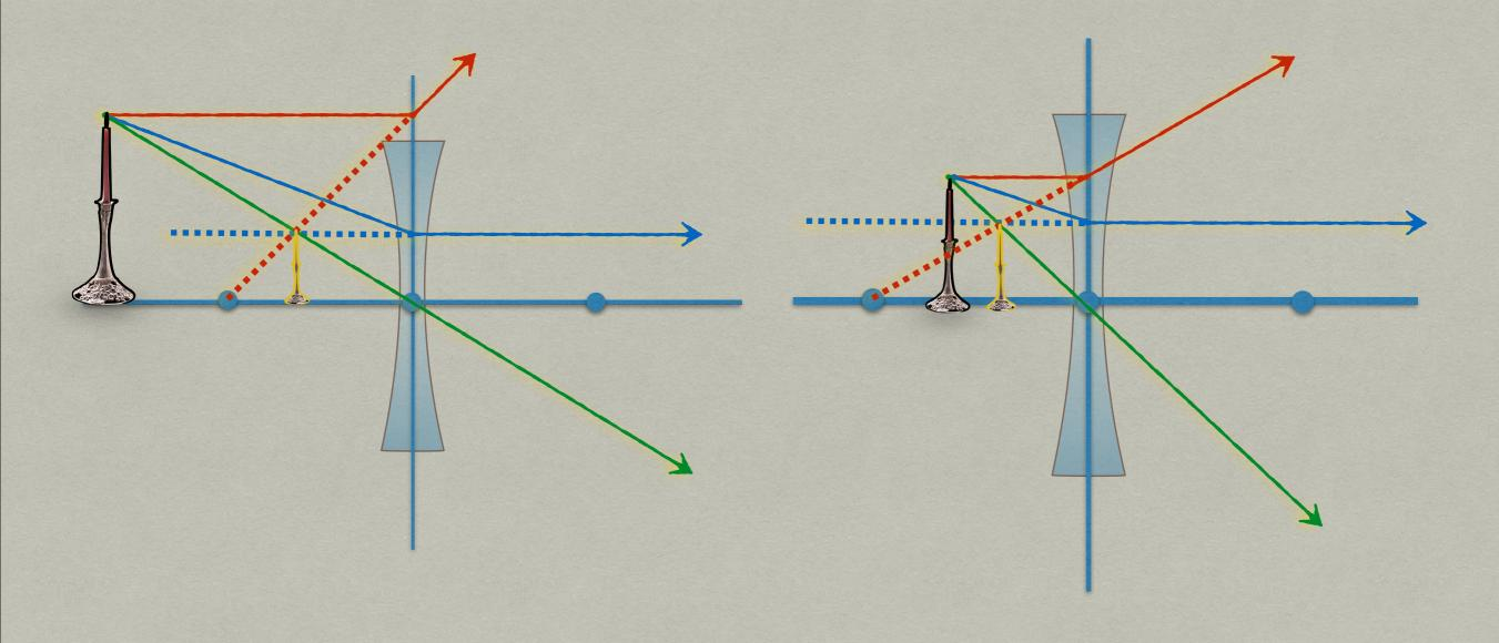
the image is similar with the object on either side of the focal point
