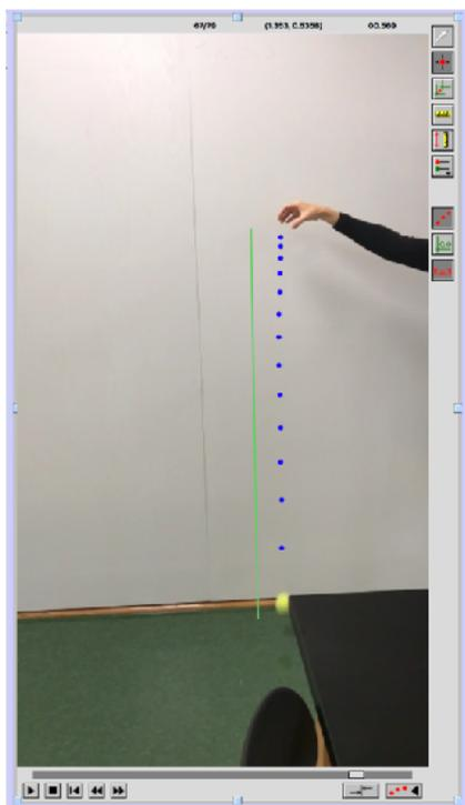
The Logger Pro software also allows for an interpretation of the motion of an object recorded with video. With a little care to keep the camera stationary, and a good reference point, you can get great results.
