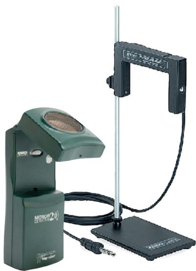
In this experiment, you may use one of two accepted methods. The first, is to use the **motion sensor** and have it graph the position of a falling object. If you choose this method, you must decide which object to drop as well as how far to allow it to fall. The second method is to use a **photogate** and picket fence combination. This method simplifies your decisions, however it only records a few data points.
